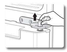
3. Remove the Middle Hinge connected to the Freezer.
